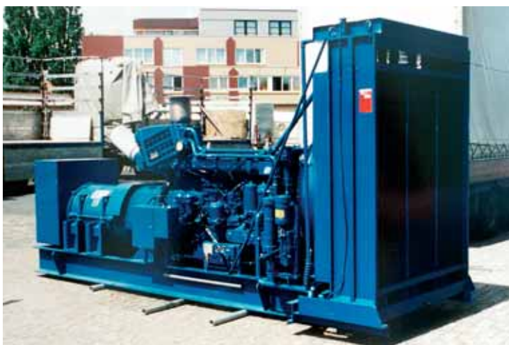
Deutz diesel engine with Leroy Somer generator
