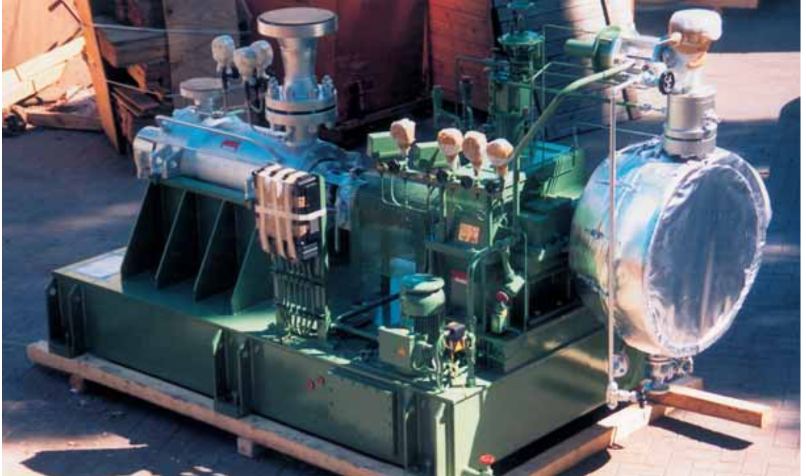
Steam-turbine-driven multistage centrifugal pump barrel-design acc. to API
