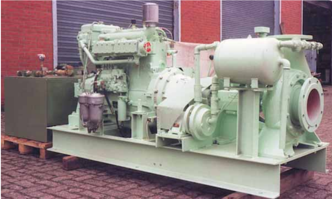
Diesel driven centrifugal pump with automatic operating evacuation system
