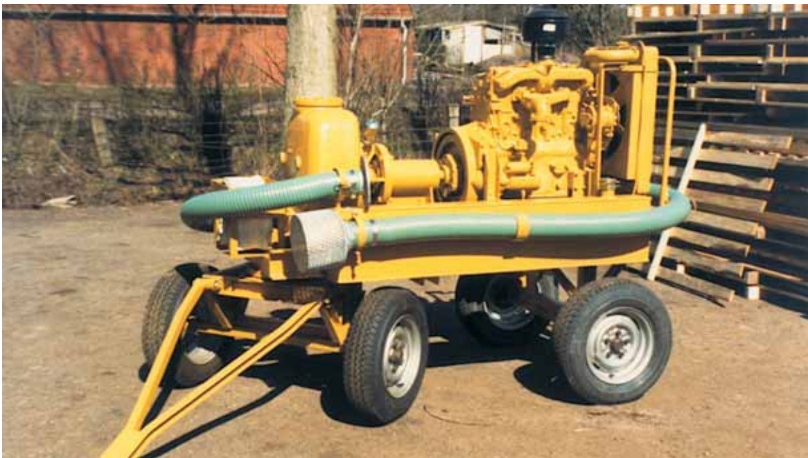
With selfpriming pump for water containing sand and solids in suspension
