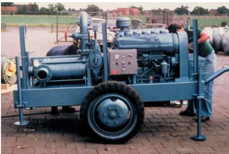
Mobile irrigation unit with multi-stage centrifugal pump and diesel engine with manual pump for evacuating
