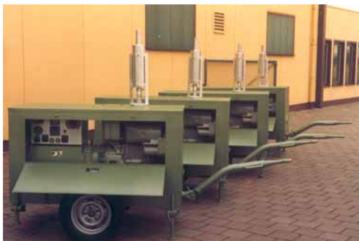
Mobile diesel-driven welding sets
