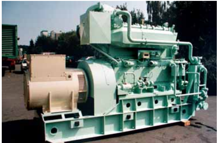
Mirrlees Blackstone diesel engine with Ansaldo generator
