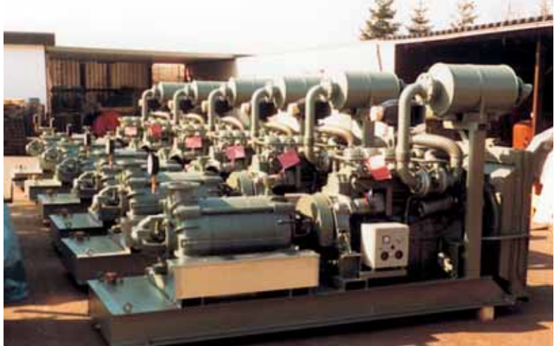
Stationary irrigation units with Mercedes diesel engines
