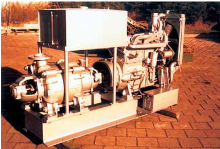
Stationary irrigation unit with self-priming centrifugal pump and diesel engine
