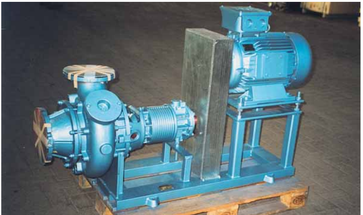
Sewage pumps V-belt driven for better adjustment
