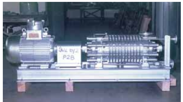
Pump with heating coil and flame proof motor for refinery
