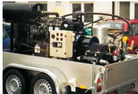
Mobile driven reciprocating pump 190 l/min - 220 bar
