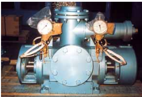
Horizontal design with temperature control for the bearings
