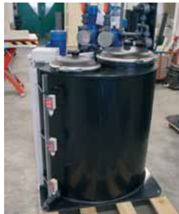
Aluminium Sulphate solution dosing compact units
