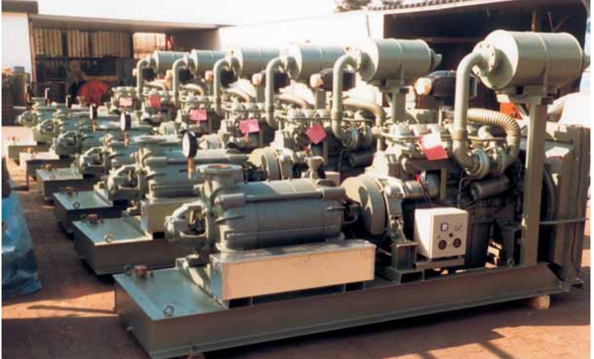
Diesel engine driven axial split-case centrifugal pumps
