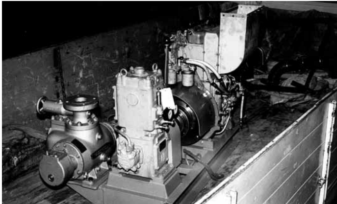
Marine diesel engine with high pressure compressor and cargo screw pump with clutch
