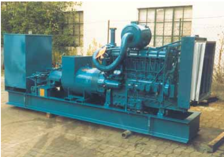
Marine diesel engine with generator and hydraulic power package
