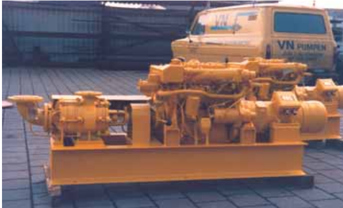
Marine diesel engine with generator and self priming fire extinguishing pump, with clutch
