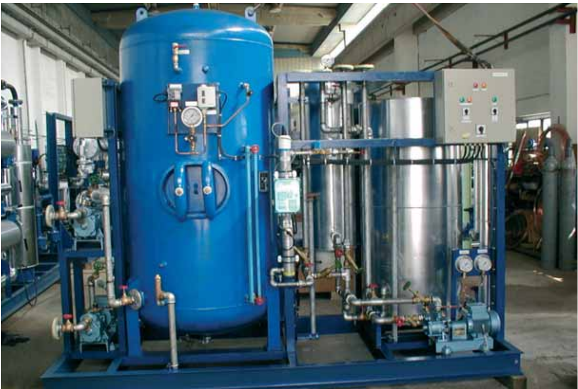
Compact units consisting of hydrophore, filter, sterilization and calorifer
